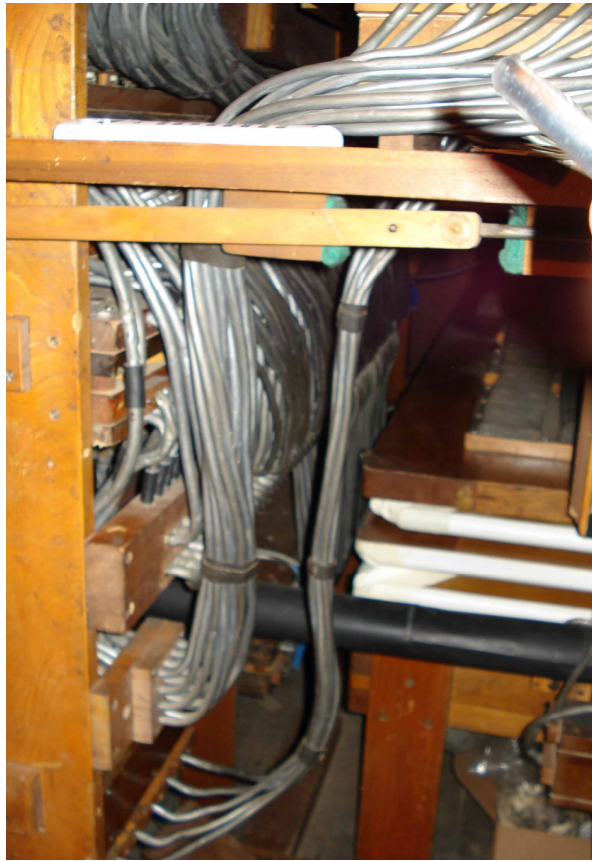
Back of the keyboard – Many of lead tubes ( \frac{1}{4} inch diameter), approximately 165 tubes, from the coupler mechanics to the wind chests; large bellows (with 3 white strips of leather), wooden rod (with green on it) controlling the crescendo level.
