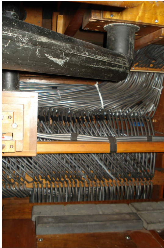
Back of the keyboard – Tens of lead tubes going to the Swell Chamber. 🎵
