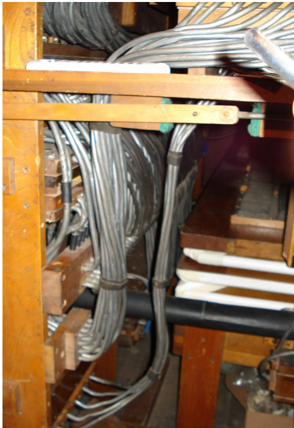
Back of the keyboard – Many of lead tubes ( \frac{1}{4} inch diameter), approximately 165 tubes, from the coupler mechanics to the wind chests; large bellows (with 3 white strips of leather), wooden rod (with green on it) controlling the crescendo level.
